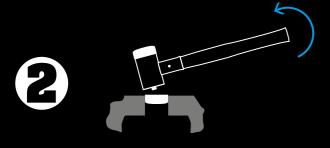
When the insert is loosened, pull the mallet upwards.
