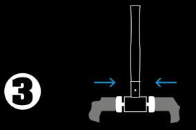
In the vice, press the new insert into the housing and insert retaining pins.
