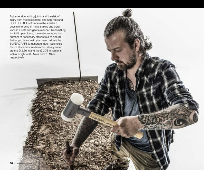
DRIVING IN REBAR / METAL STAKES
