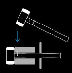
Tap the clamping pin into the bore hole.
