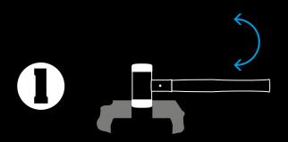
Firmly clamp the used insert in a vice and loosen with a lateral twisting movement.
