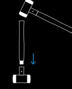
Tap an aluminium wedge into the slot found in the wooden handle.
