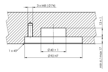
Mounting depth Connecting Element and Connecting Ring:
