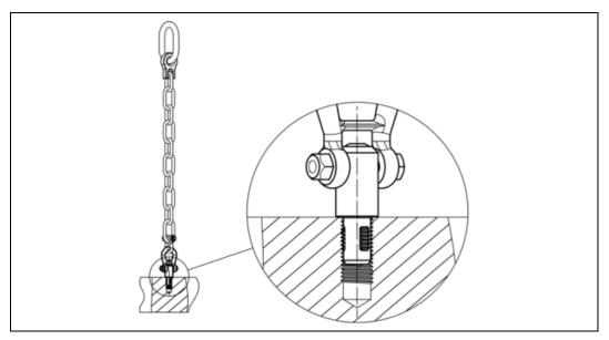
Figure 4: Installation examples - threaded lifting pins, self-locking
