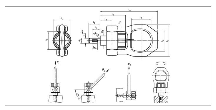
Figure 11: Dimensioned drawing - threaded lifting pins, self-locking, with rotatable shackle - EH 22353
