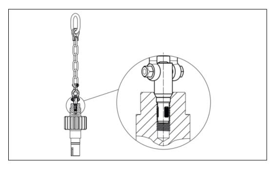
Figure 5: Installation examples - threaded lifting pins, self-locking, for centre holes according to DIN 332
