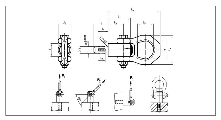
Figure 9: Dimensioned drawing - threaded lifting pins, self-locking - EH 2B352
