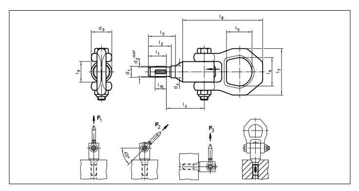
Figure 10: Dimensional Drawing - threaded lifting pins, self-locking, for centre holes according to DIN 332
