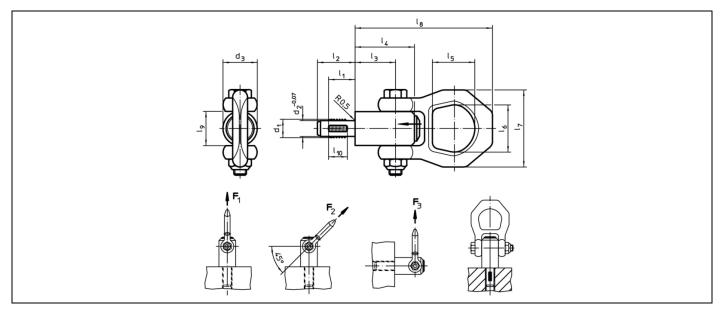
Figure 8: Dimensioned drawing - threaded lifting pins, self-locking - EH 22352
