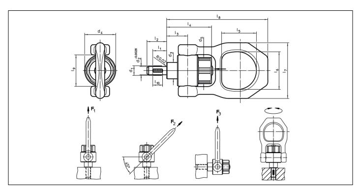
Figure 12: Dimensioned drawing - threaded lifting pins, self-locking, with rotatable shackle - EH 2B353
