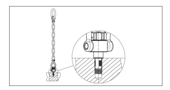
Figure 6: Installation examples - threaded lifting pins, self-locking, with rotatable shackle
