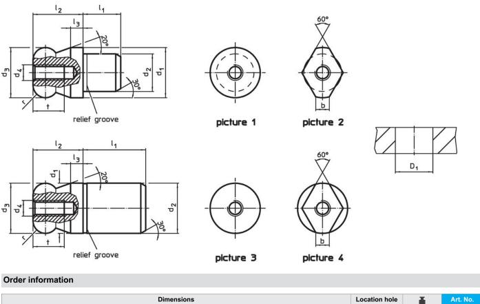
T D<sub>1</sub> d<sub>1</sub>  $d_2$ d<sub>3</sub>  $d_4$ b I<sub>1</sub> l<sub>2</sub> I<sub>3</sub> H7 n6 -0.01 g6 -0.05 [g] [mm] [mm] with ball end flattened - picture 2, Tool steel 22630.0412 12 8 12 M4 8 12 3 8 3 2.5 8 8
