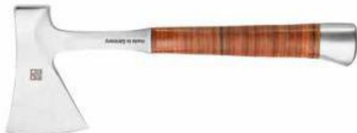
Robust all-metal design made from special heat-treated steel, forged in one piece, finely ground and polished on all sides, corrosion-resistant, blade carefully hardened and ground to sharpness, hand-made, anti-slip leather handle, perfectly balanced for optimum handling
