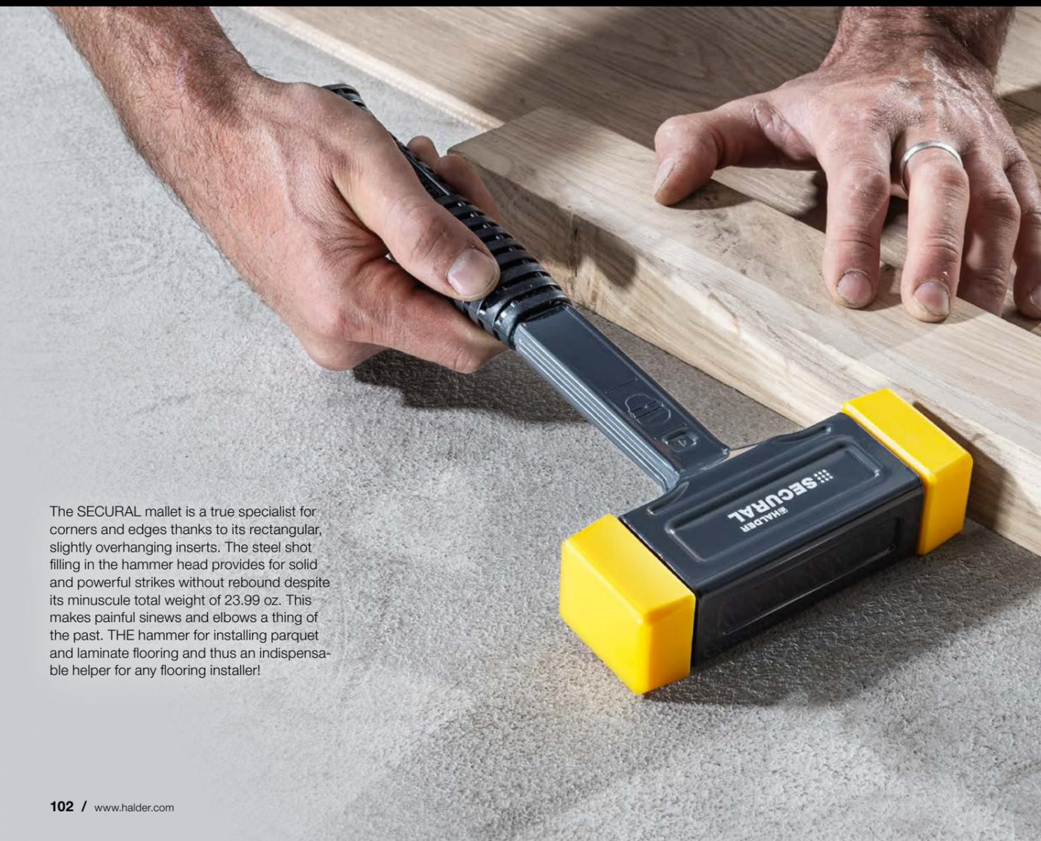
The SECURAL mallet is a true specialist for corners and edges thanks to its rectangular, slightly overhanging inserts. The steel shot filling in the hammer head provides for solid and powerful strikes without rebound despite its minuscule total weight of 23.99 oz. This makes painful sinews and elbows a thing of the past. THE hammer for installing parquet and laminate flooring and thus an indispensable helper for any flooring installer!
