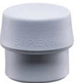
A thermoplastic elastomer, the SIMPLEX insert TPE-mid boasts a hardness of approx. 90 Shore A, making it an insert of medium hardness (comparable to the hardness of the rubber composition insert included in the 3202 series). Unlike conventional rubber mallets, this grey insert does not leave behind any undesired black marring.
