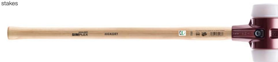
Wooden stakes will splinter if driven in with steel hammers or soft-face mallets whose head diameter is too small. This is why HALDER offers the SIMPLEX sledge hammer with superplastic inserts and an extra large diameter of 4.92 in. The non-rebound forestry sledges deliver increased impact force, while their completely flat nylon inserts prevent the stakes from splintering.
