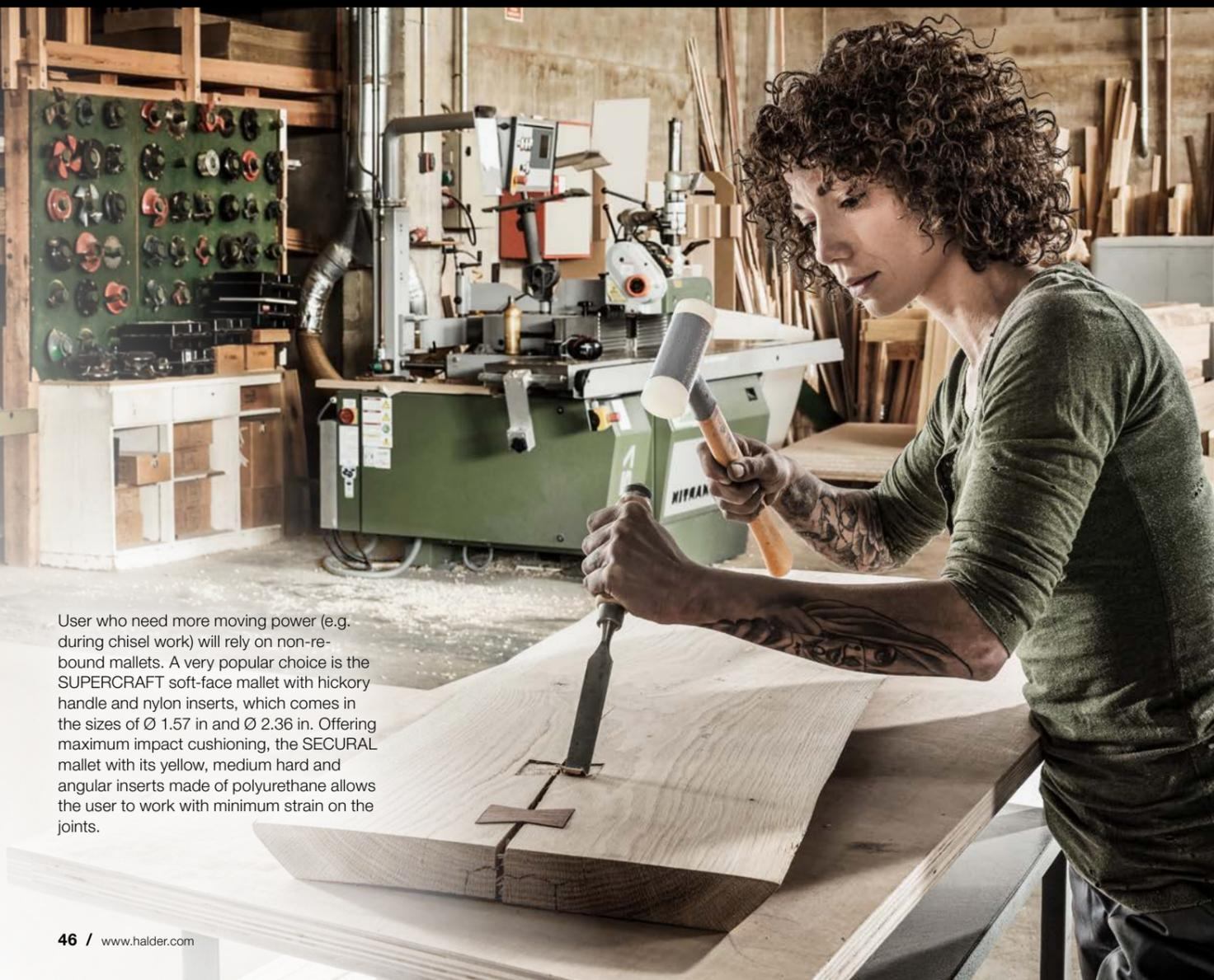
User who need more moving power (e.g. during chisel work) will rely on non-rebound mallets. A very popular choice is the SUPERCRAFT soft-face mallet with hickory handle and nylon inserts, which comes in the sizes of Ø 1.57 in and Ø 2.36 in. Offering maximum impact cushioning, the SECURAL mallet with its yellow, medium hard and angular inserts made of polyurethane allows the user to work with minimum strain on the joints.
