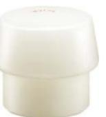
With its hardness of approx. 73 Shore D, the SIMPLEX insert Nylon is an extremely hard insert. This white polyamide insert offers outstanding impact qualities and is guaranteed to combine maximum strength with unique durability. It is composed of extruded and extremely homogeneous material. Compared to injection moulded plastic inserts, it is therefore considerably more wear-resistant and durable and will never chip even in sub-zero temperatures. Moreover, it is also oil and grease resistant.
