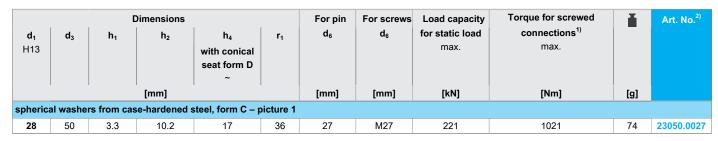
$<sup>^{1)}</sup>$  Torques of screws with standard thread, eventual pre-loads to be considered, coefficient of friction  $\mu_{total}$  0.14.
