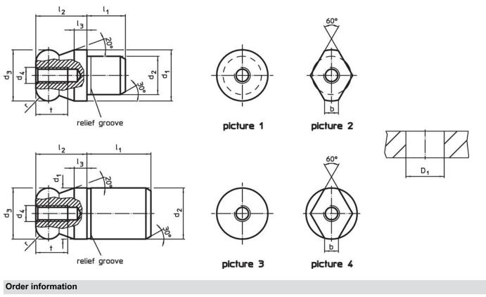
Dimensions Location hole Art. No. T D₁  $d_3$ b d₁  $d_2$ d₄  $\mathbf{I}_1$ l<sub>2</sub> 1 r H7 g6 n6 -0.01 -0.05 [mm] [mm] [g] with ball end flattened - picture 2, Stainless steel 16 12 16 M5 12 16 4 10 4 4.3 12 25 22630.0456
