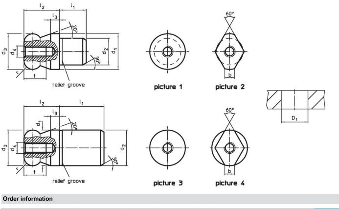
Dimensions Location hole Art. No. D₁ b d₁  $d_2$ d<sub>3</sub> d₄ h 12 I<sub>3</sub> H7 g6 n6 -0.01 -0.05 [g] [mm] [mm] with ball end flattened - picture 2, Stainless steel 12 12 M4 8 12 3 8 3 2.5 8 8 22630.0452 8
