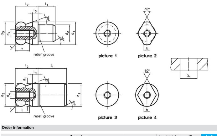
Dimensions Location hole Art. No. Т D₁  $d_2$ d<sub>3</sub> d₄ b d₁ h b I<sub>3</sub> t r H7 g6 n6 -0.01 -0.05 [g] [mm] [mm] with ball end flattened - picture 2, Stainless steel M2,5 2 4.5 1.7 4 1.5 22630.0446 6 4 6 4 6 1
