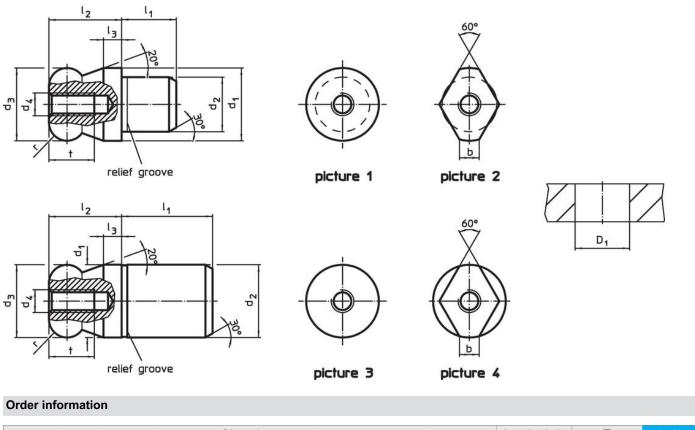
Location hole Dimensions Art. No. Т D<sub>1</sub> d3 d₁  $d_2$  $d_4$ l<sub>2</sub> h I<sub>3</sub> t r H7 g6 n6 -0.01 -0.05 [mm] [mm] [g] with ball end plain - picture 1, Tool steel 6.7 22630.0310 10 10 М3 7 10 2.5 6 2.5 7 7
