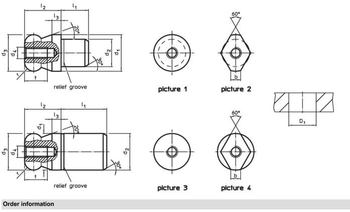
Location hole Dimensions Art. No. Т  $D_1$  $\mathbf{d}_3$ d₁  $\mathbf{d}_2$  $\mathbf{d}_4$ I<sub>1</sub> l<sub>2</sub> I<sub>3</sub> t r H7 g6 n6 -0.01 -0.05 [mm] [mm] [g] with ball end plain - picture 1, Tool steel 22630.0308 8 М3 6 8 2 6 2 6 3.9 6 8
