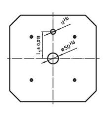
$^{\ast}$  These tolerances are valid only for optional exterior stop type. Slot spacing 70 ±0,01.
